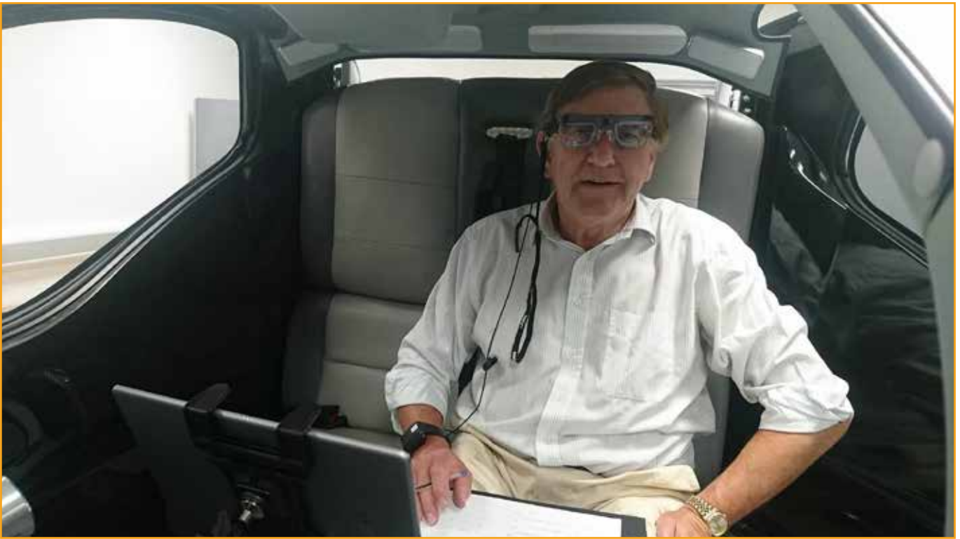
Figure 4 - Tobii Eye Tracking Pro 2 Glasses inside Simulator
