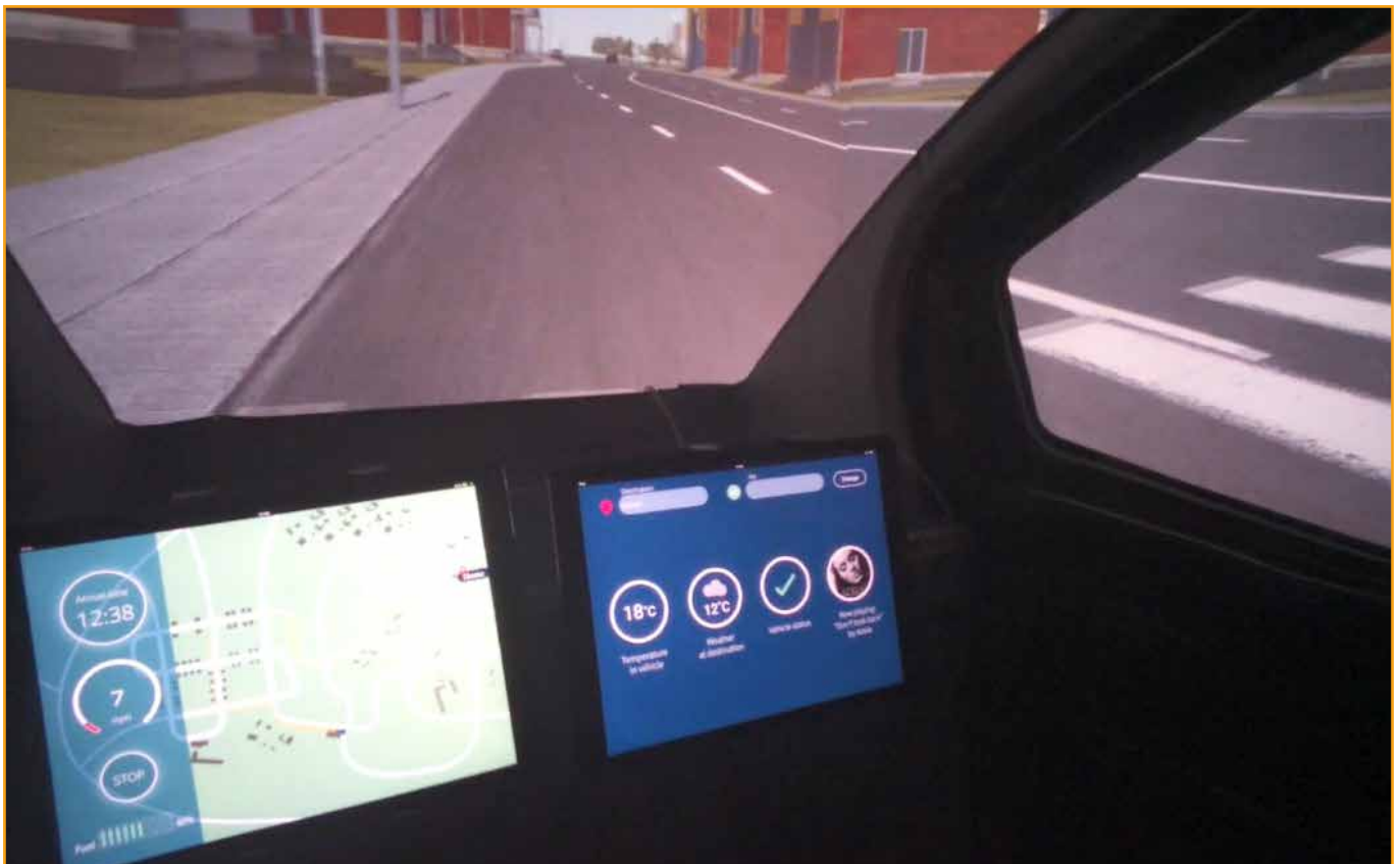
Figure 6 - Simulator Trial 2 HMI – showing two-screen interface
