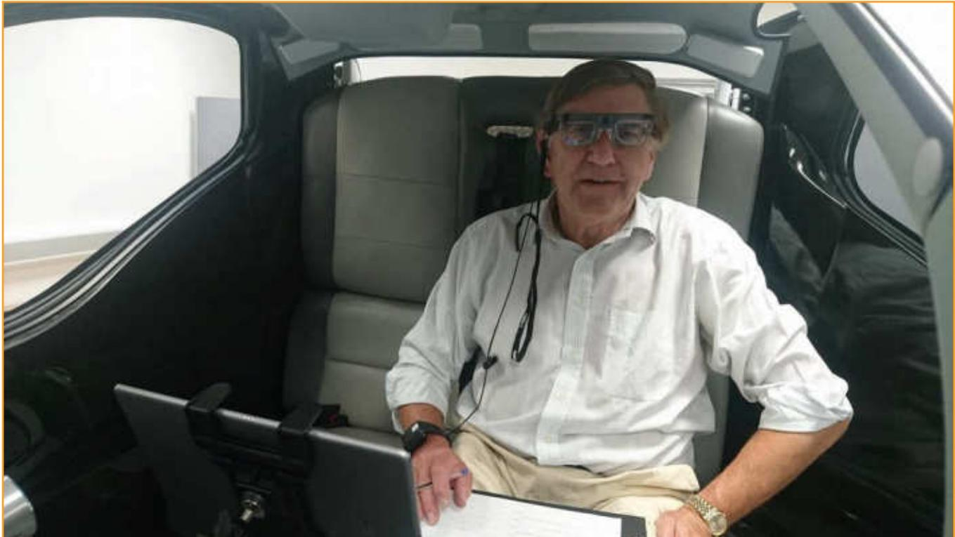
**Figure 4 - Tobii Eye Tracking Pro 2 Glasses inside Simulator Trial 1**
