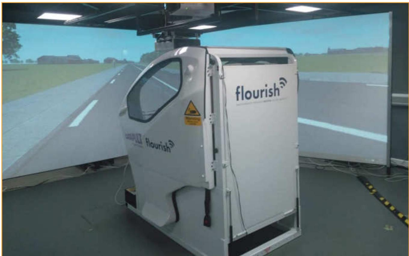
**Figure 5** - Exterior of the pod used in Simulator Trial 2, including large wraparound screens
