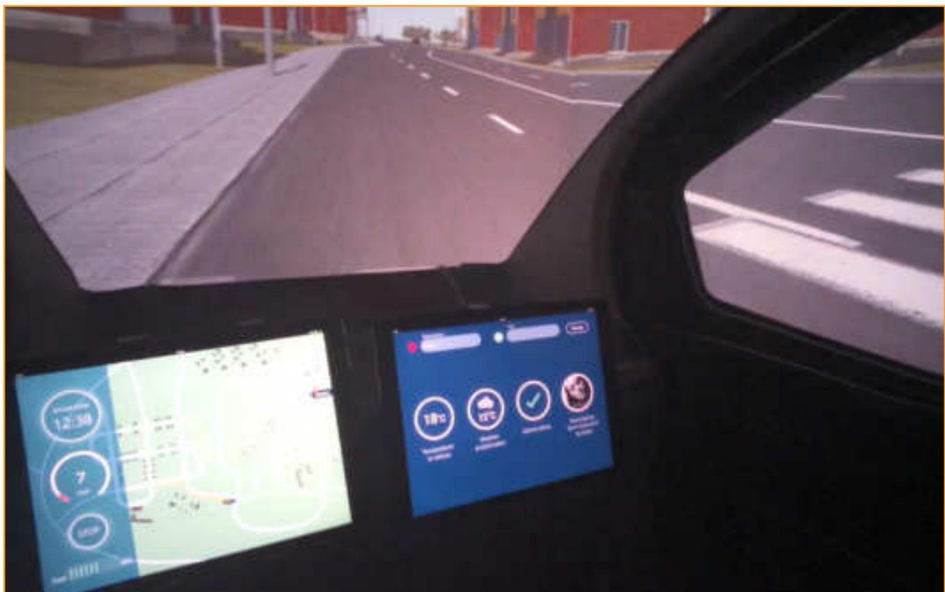
**Figure 6** - Simulator Trial 2 HMI – showing two-screen interface
